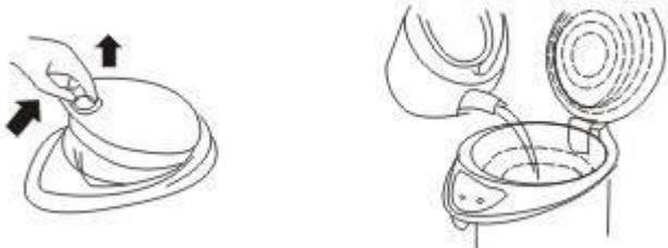
Press the lid opening switch to unlock the lid's top cover and open it.
